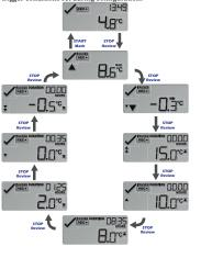
These screens show each configured alarm threshold temperature, and the time recorded during the trip above this temperature, in descending order.
