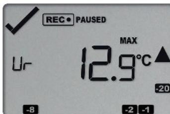
Pressing the **REVIEW/MARK** button
