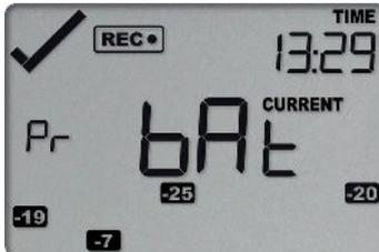
Figure 8: Probe Low Battery screen
