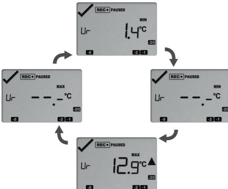
During the cycle, the buzzer will sound a series of short beeps.
