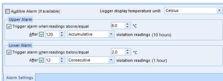
Figure 2: Sample Alarm Configuration Settings for a TRED30-16
