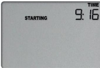
Once **READY** disappears, release the button within two seconds. **STARTING** will also disappear, and the **REC•** symbol will be shown. The TRED30-16 now records temperature data.
