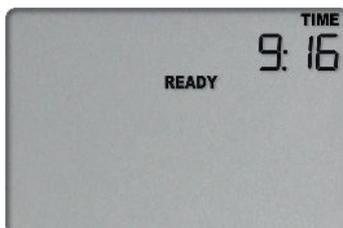
Press and hold the **START/CLEAR/STOP** button. First, **STARTING** is shown in addition to **READY**:
