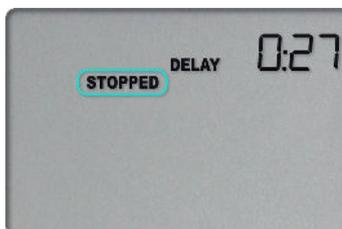
**STOPPED** and **DELAY** will both disappear, and **READY** will show, together with the current time, and the logger can now be started again as normal.
