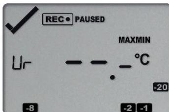
Release the **REVIEW/MARK** button when the screens no longer alternate. The values will be reset, and the normal recording screen will be shown.
