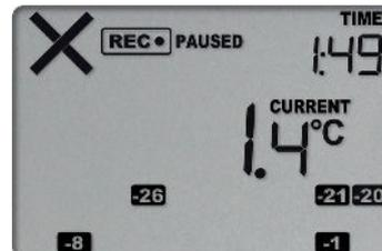
In this example the paused function was activated, and the paused symbol is shown on the display. For more information about paused readings please see the section about [Paused Readings below](#).
