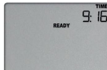
If the button is released while **STOPPED** is still blinking, or you wait until the **READY** symbol disappears, the display shows **STOPPED** again, and the logger remains stopped. This means, the data from the previous trip is still accessible.
