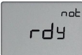
To use the logger again for recording data, it must be re-configured with LogTag Analyzer.
