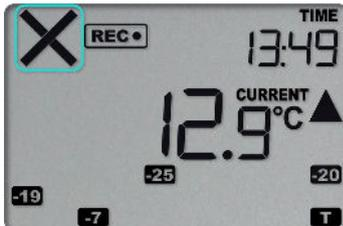
Each alarm trigger condition consists of a threshold temperature value, an activation type (which can be instant, consecutive or accumulative<sup>2</sup>) and a delay time, if it is not an instant alarm.
