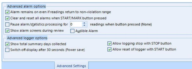
*Figure 3: TRED30-16 advanced configuration screen in LogTag Analyzer 3*
