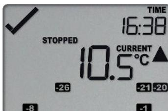
Release the button within 2 seconds. The logger will now stop taking readings.
