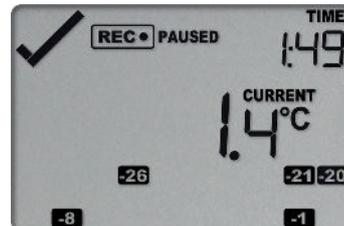
A mark will be placed in the readings when you clear an alarm.
