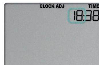
Accept the hours value by pressing
