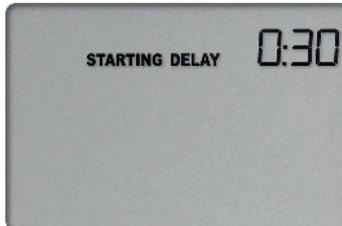
The delay time is shown in hours and minutes. The time counts down and the TRED30-16 starts recording when it reaches **0:00**.
