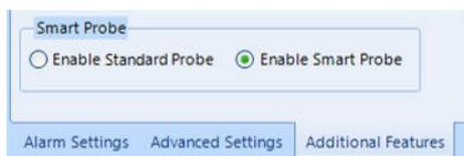
When used with the standard analogue probe, the system must be calibrated as a whole (logger and probe).
