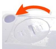
You can use the new battery for this, as it will fit into the slot
